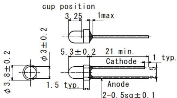
**Figure-14  $\Phi 3$ Mold (Type36)**
