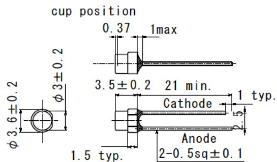
**Figure-12  $\Phi 3$ Mold (Type33)**
